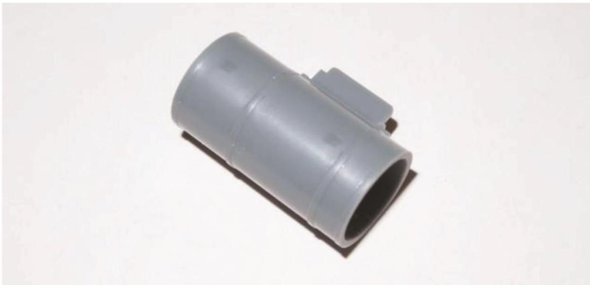
Now this is a very important step – do not neglect it! Drill a small diameter hole through the cylinder from outside to inside. I locate the hole in the mounting tab so it won't be seen and won't need clean up later. I discovered this the hard way. Epoxy cures with a thermal reaction that heats up the air trapped inside the cylinder. The expanding air
