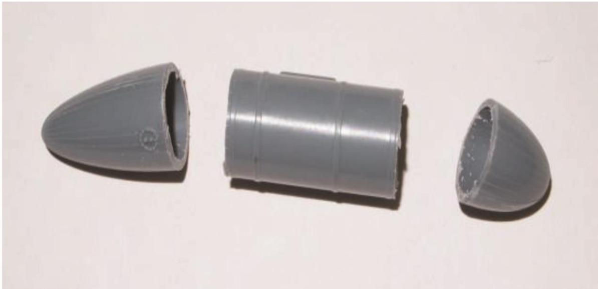
Next carefully trim the waste away and clean up the ends so they are nice and square. I use my lathe for this step but it can be done with a flat file – choose one that is wide enough to cover the full diameter. Also, I found that removing the alignment pin protrusions on the inside helps avoid any interference with the resin parts.
