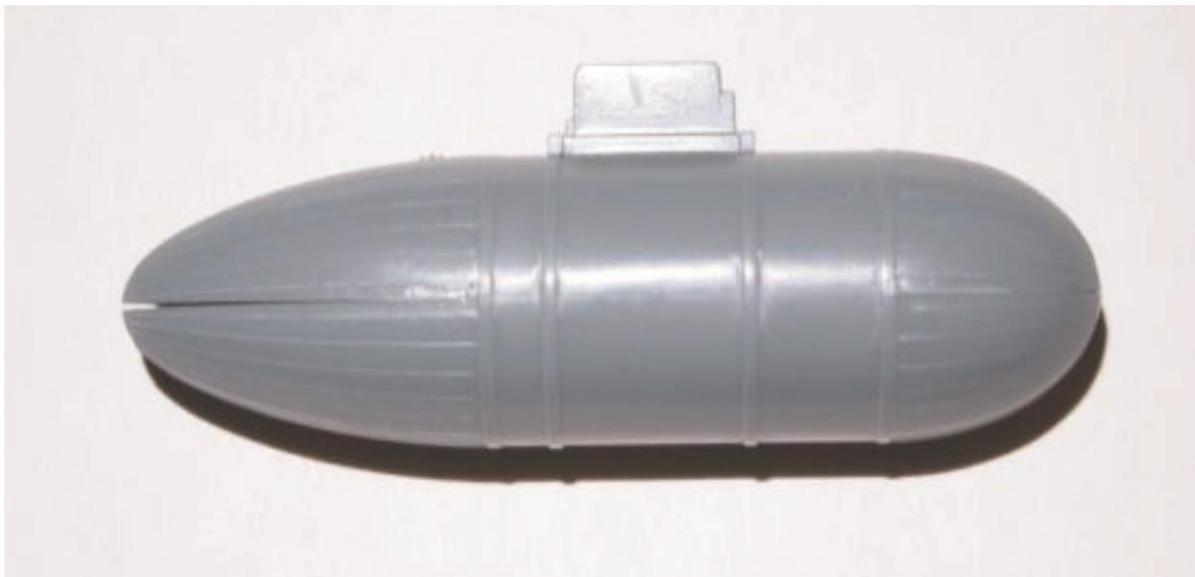
Now, cut off the nose and the tail. I use a razor saw and leave a little “waste” for final clean up ahead and behind the front and rear straps.
