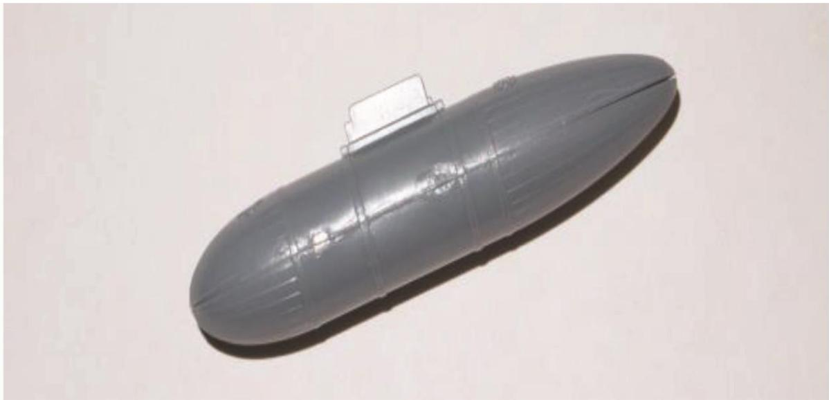
The next step is to clean up the seams like any seam work done on a plastic model. I like to use a Flexi-file with a sanding strip that has been thinned to easily fit between the closest straps near the tail. Then I polish out any scratches with fine grit sanding pads.
