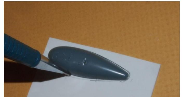
7. Using one half, trace the outline on a piece of 0.015" thick plastic sheet. The outline should be about 0.015" larger than the tank half all the way around the perimeter.
